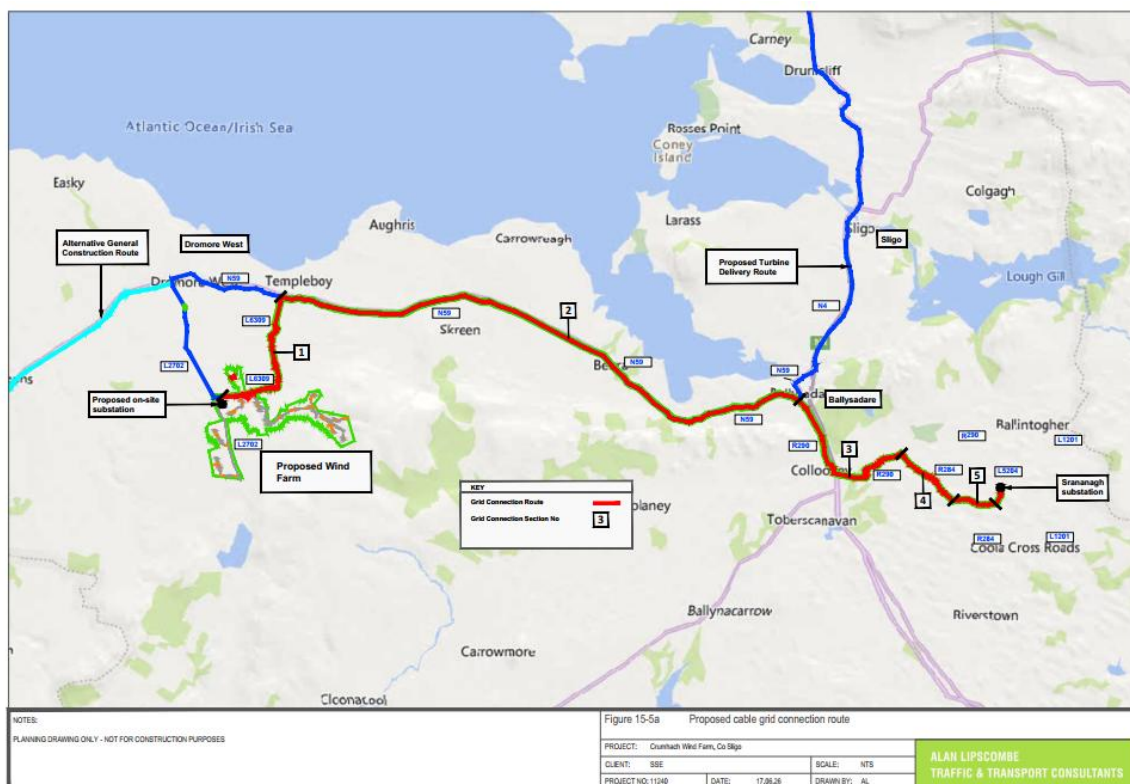
Figure 15-5a of EIAR - Proposed cable grid connection route
